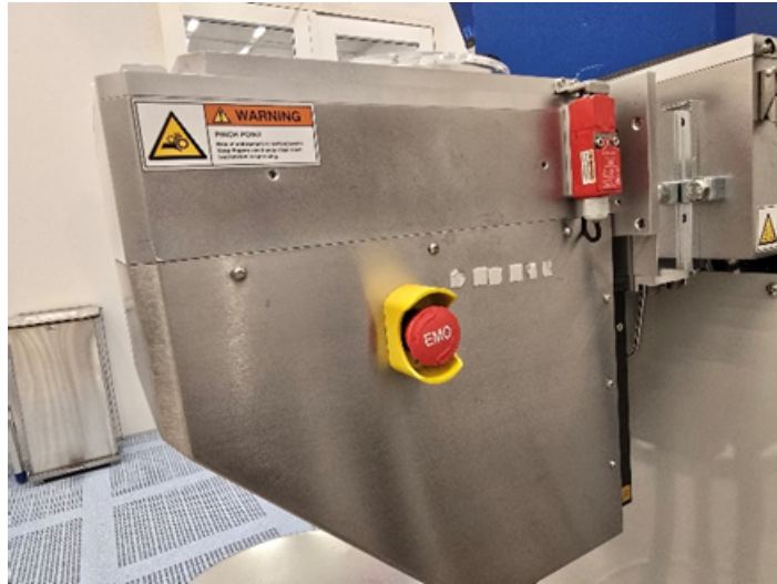
Image 12 EMO located at the side wall of the load lock chamber
