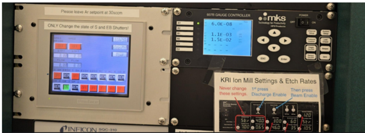
Figure 15: An example of what the idle state should look like before you leave the tool – you do not need to wait around until the chamber pressure gets very low.
