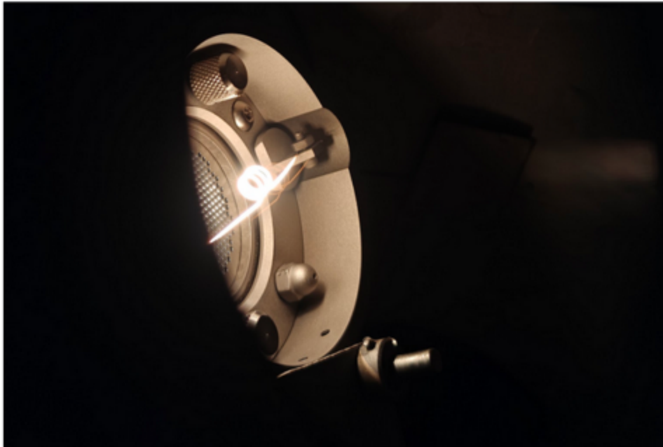
Figure 13: Ion milling filament when setup properly.
