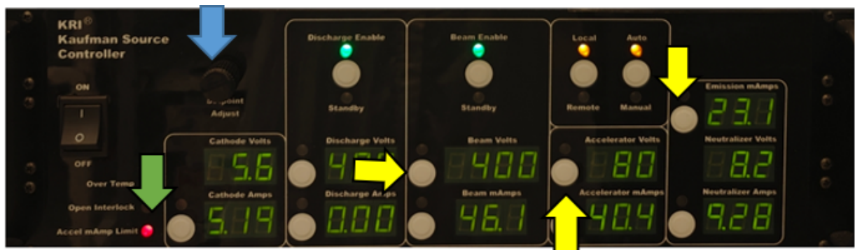
Figure 12: Blue arrow shows the knob is to adjust parameter value. Yellow arrows represent where the parameter adjustment button is. The green arrow shows the red LED light that could turn on during use.
