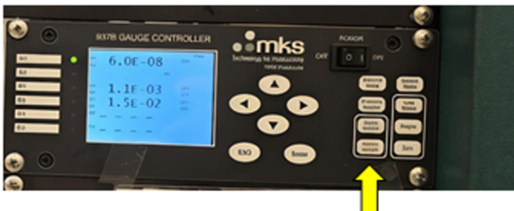
Figure 8: Yellow arrow shows where the sensor on/off is located.
