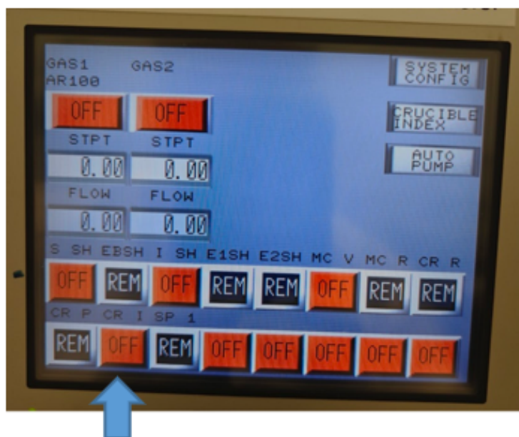
Figure 9: Blue arrow shows where the top cryo button (Cr_I) is located. OFF represents closed.
