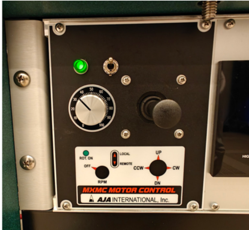
Figure 14: Green LED is on, which represents it's spinning. The toggle switch is in the UP position which is LOCAL mode.
