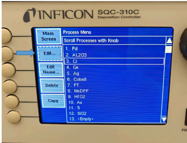
Figure 6: After you press the “Process Menu” button, it takes to this screen to select a material. Choose the material you will be depositing, and in order to make the selection (or move on to the next screen), you must press it twice.
