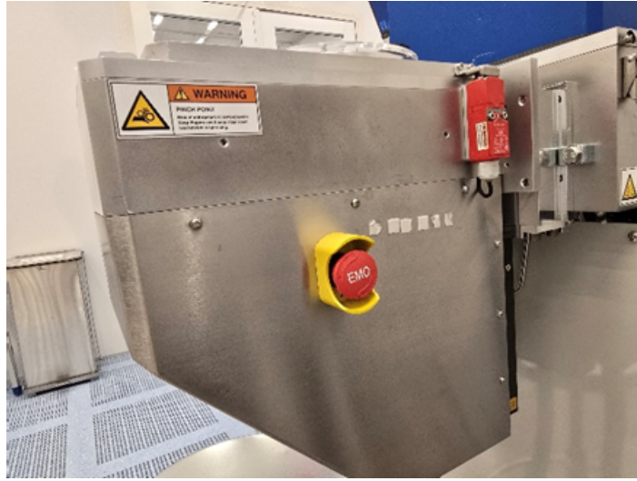
Image 3 EMO located at the side wall of the load lock chamber
