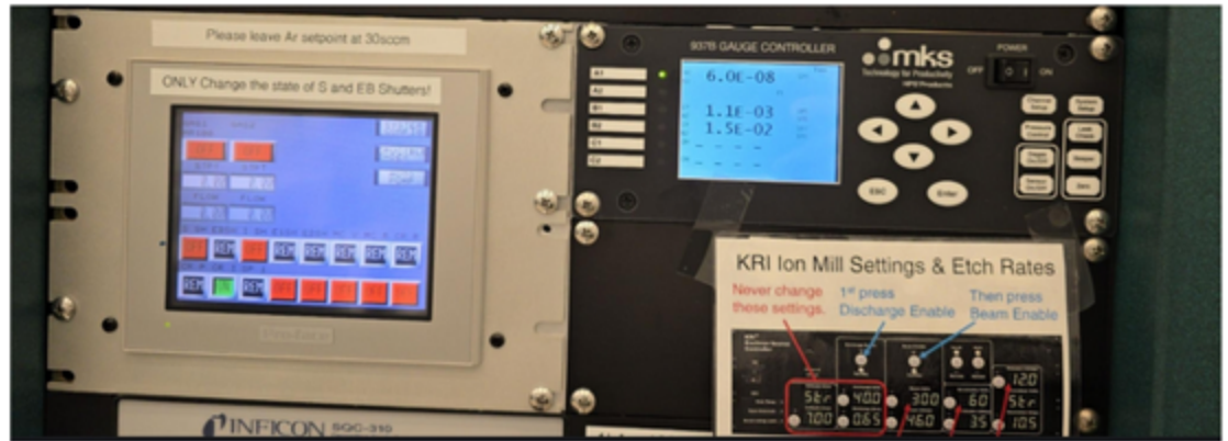
Figure 13: An example of what the idle state should look like before you leave the tool – you do not need to wait around until the chamber pressure gets very low.
