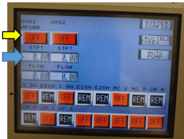
Figure 10: Blue arrow shows where to edit the gas flow. Yellow arrow turns On/Off the Ar gas.
