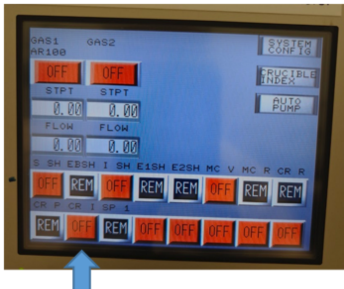
Figure 9: Blue arrow shows where the top cryo button (Cr_I) is located. OFF represents it's closed.
