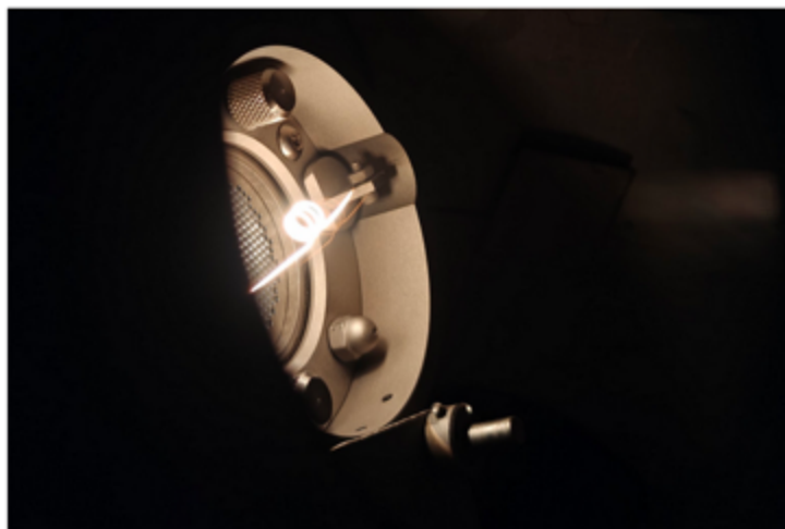
Figure 13: Ion milling filament when setup properly.
