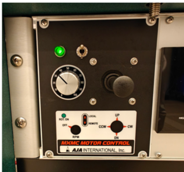
Figure 14: Green LED is on, which represents it's spinning. The toggle switch is in the UP position which is LOCAL mode.
